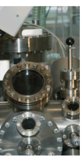
Empa researcher Andreas Züttel is "producing" CO<sub>2</sub>. The physicist uses the vacuum analysis equipment in the background to investigate how CO<sub>2</sub> and H<sub>2</sub> can bond together on metal hydride surfaces to form olefins, the basis for synthetic fuels. His vision: to create fuel from the greenhouse gas CO<sub>2</sub>.
