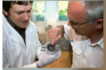
PhD student James Shaw-Stewart (left) and project manager Matthias Nagel examine the completed chip. On the plate, which is enclosed in a protective atmosphere, pixels should start glowing in three colours. If they do, the experiment was a success.
