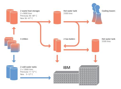
Air conditioning system in the Swiss IBM head office: 25 per cent less energy consumption without structural changes. Right: IBM Switzerland head office in Altstetten.
