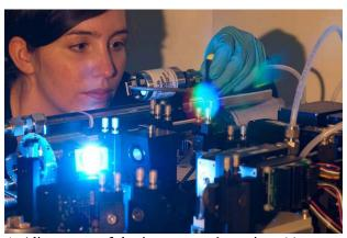
4. Alignment of the instrument's optics: this operation is critical because the sensitivity of measurement is dependent upon this alignment.
