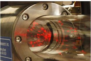
7. Measuring chamber: The gas sample to be evaluated is introduced continuously (up to 10 liters/minute) and is measured through the absorption of the laser beam (visible in red on this image). The absorbed photons do not continue on the path towards the detector and are thus counted as "void", translating the presence of the corresponding gas molecule.
