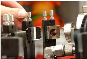
6. Precision alignment of the optics: The laser beam must be guided towards the measuring chamber, and then the signal is turned towards the detector. This requires a perfect control of the optical path using specialized mirrors and lenses.
