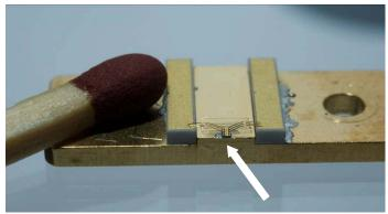
3. The quantum cascade laser (QCL). The laser beam is emitted by the divice indicated by the arrow.
