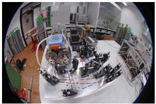
8. Other views of the optical instrument: the optical path is indicated by dotted lines on the optical table because the laser beam is in fact invisible (infra-red light)
