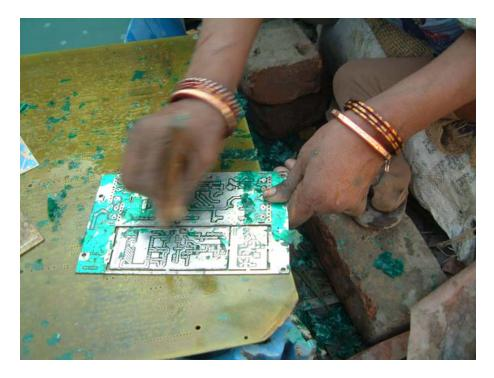
The unprofessional disassembly of electronic devices at the end of their useful life – as in this case in India, where copper is being removed from a PCB – represents a danger to human health and the environment.
