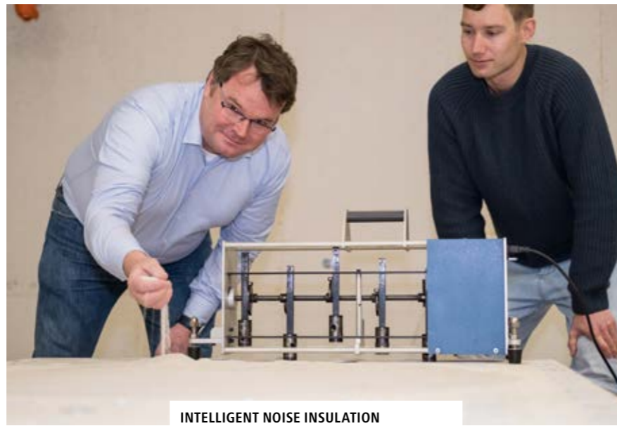
INTELLIGENT NOISE INSULATION Stefan Schoenwald and Sven Vallely verify whether the vibrations of the real wooden panel correspond to the calculations (coloured image below). The cavities are now filled with sand, which converts the vibrations into heat. A "footfall sound simulator" knocks on the panel with metal hammers.
