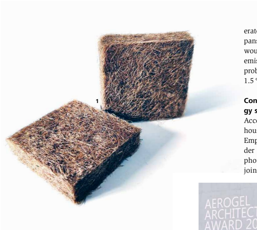
1 Insulation panel based on fibers from algae washed up on Mediterranean beaches and typically disposed of as waste.
