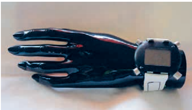
Prototype of the “blood-pressure watch” with the Empa strap made of piezo-resistive fibers.
