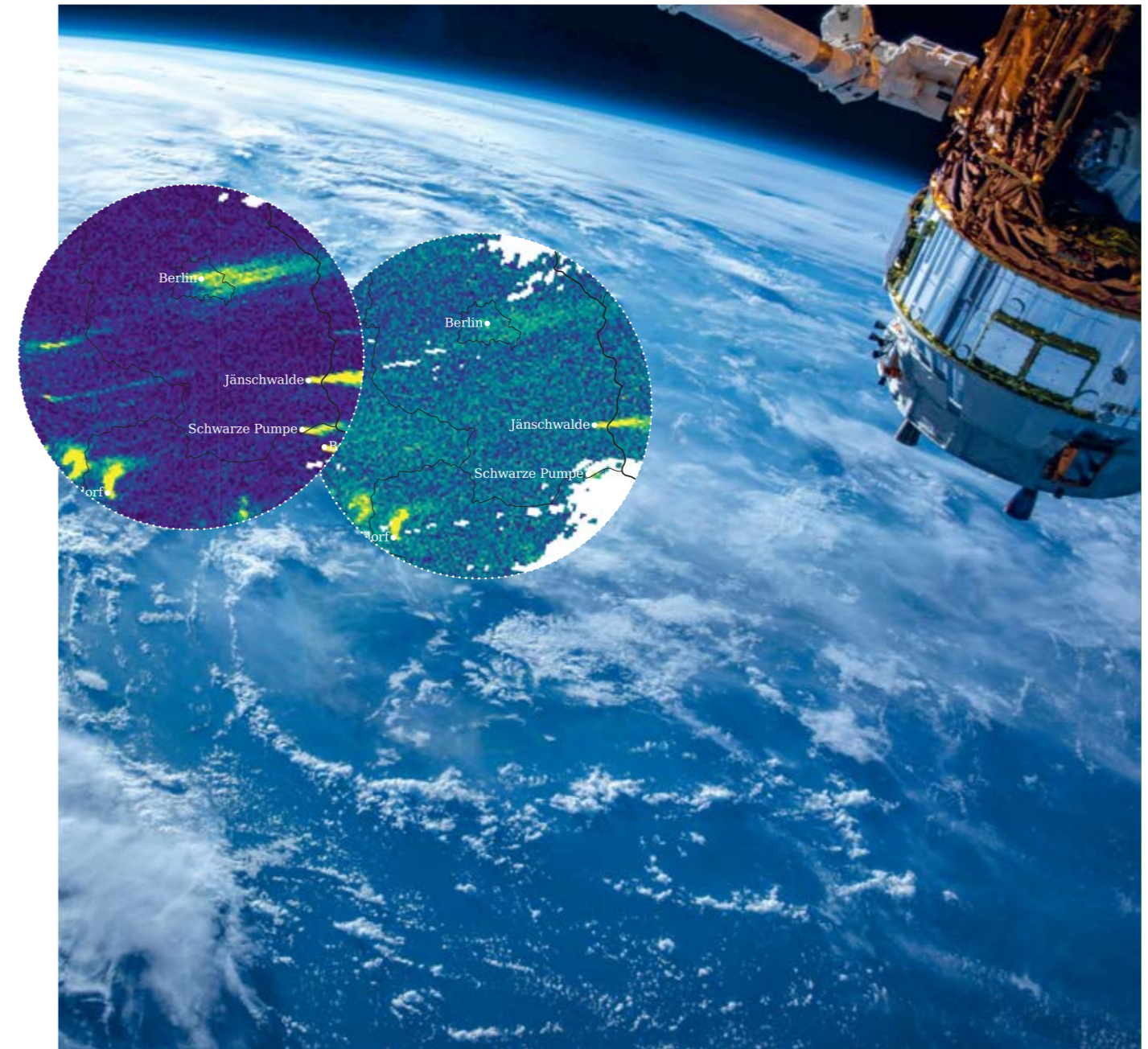
Satellite images from Empa researchers’ simulations: in areas where high NO 2 values (right) coincide with high CO 2 values (left), the high levels of CO 2 are man-made. The emissions of the city of Berlin and several coal-fired power plants are clearly visible. The aim of the EU and ESA is to detect CO 2 emissions almost in real time in order to be able to reliably and promptly determine greenhouse gas emissions worldwide in the future. Image: Unsplash/NASA
