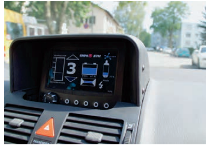
Display monitoring the vehicle condition (right). The CLEVER car – Empa's natural-gas fuelled hybrid research automobile based on the VW Touran.
