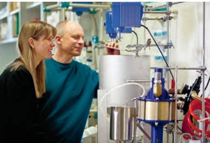
The conversion of cellulose into the high-tech product NFC begins in a metal funnel. Here two Empa researchers investigate the properties of the material.
